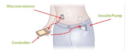
Artificial Pancreas System. A sensor measures glucose levels and transmits them to a mobile-phonesized controller, which runs a control algorithm. An insulin pump delivers insulin subcutaneously. The communication is wireless. Reprinted from Hovorka, Nature Reviews Endocrinology, 2016.
